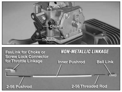
**5.** Install the throttle servo and choke servos at least 12" [305mm] away from the engine. Make sure that you get the throttle and choke's full range of rotation with your servos travel. Be sure to use a non-metallic linkage for both the throttle and choke linkage. A high-torque heavy duty metal gear servo is recommended to operate the throttle on the DLE-170. (Components for the non-metallic linkage can be purchased through your local hobby shop.)
