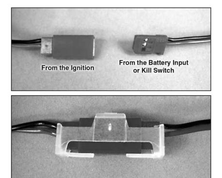
**3.** Connect the ignition kill switch lead to the red connector from the ignition control module using the lead from the kill switch or with the included three pin connector with pig tail. Use the included three pin securing clip to secure the connection.
