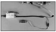
Many of the DLE Ignition modules have an additional lead to plug into the optional tachometer. If your ignition module does not have this additional lead, the digital tachometer can still be used. Simply use the Y-harness
