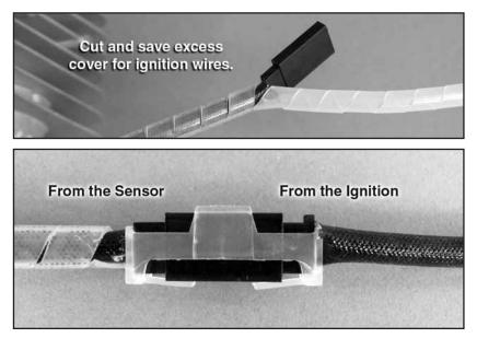
**2.** Install the silicone wire cover over the pick up lead coming from the engine (cut the excess silicon wire covers) and connect the lead to the pick–up lead from the Electronic Ignition Module. Secure the connection with the included three pin connector securing clip.
