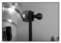
8. Install a 2-56 ball links (not included) to the throttle & choke control arms. Use a 2-56 lock nut to secure the ball links or use (2) 2-56 nuts and thread locker to secure the links. Once the links are secure, exercise the throttle and choke levers to ensure that no binding occurs.
