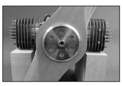
**4.** Place the propeller on the crankshaft at the one o'clock position.
