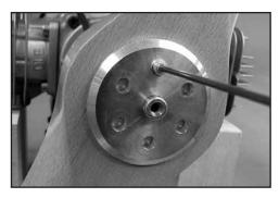
**5.** Mark the location of one of the outer holes on the propeller. Use a GPM Dead Center Hole Locator (GPMR8130) to center and start the hole.
