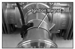
**3.** Next, set the engine near the beginning of the compression stroke. Note the position of the ignition magnet with engine inverted.
