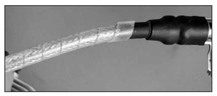
**5.** Install the silicone ignition wire cover over the ignition wires to the spark plugs.
