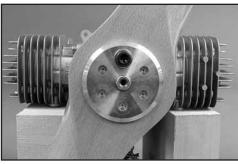
**6**. Remove the propeller from the engine and drill the outer hole on the drill press using a #35 (.110"/2.81mm) drill bit as a pilot hole. Next use a 1/4" (6.28mm) drill bit to finish the hole. In order to achieve a clean finish on both sides of the propeller drill only half way through
