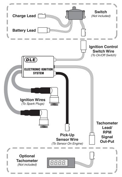
**7.** Use the above diagram to install the Electronic Ignition Module to the engine.
